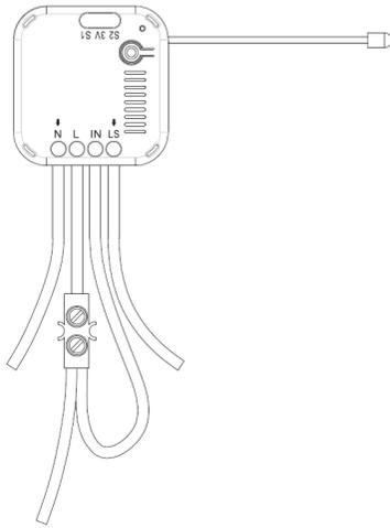
**Note:** Please use 1.25m<sup>2</sup> wires. When there are two or more wires, please use the appropriate external terminal wiring as shown above.
